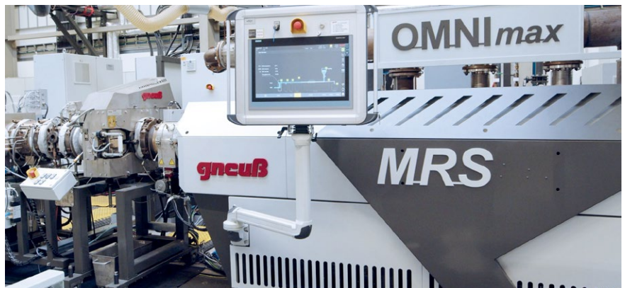
Gneuss OMNImax recycling machine with MRS extruder and RSFgenius filtration system
