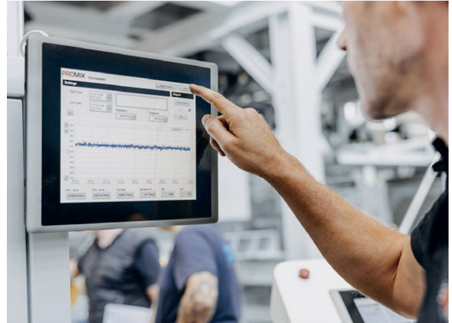
The inline viscometer "Visco-P" measures the actual viscosity of the melt under process conditions in real time (Pictures: Promix Solutions AG)
